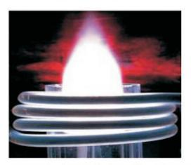
ICP inductively coupled plasma single-channel scanning spectrometer, is a multi-element analysis of the sequence test measuring equipment. The instrument consists of scanning spectrometer, radio frequency generator, the sample introduction system, photoelectric conversion, control systems, data processing systems, and analysis software. Plasma is generated from the triple concentric
